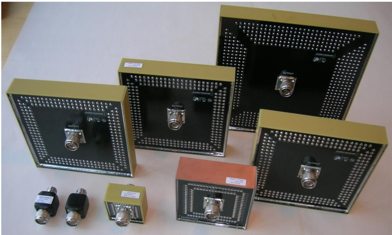
**Figure 1: A set of current shunts with nominal values ranging from 30 mA to 20 A.**
